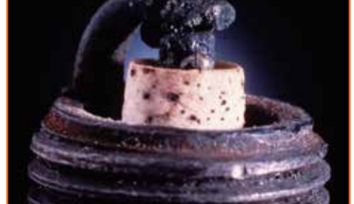
SUSTAINED PRE-IGNITION DAMAGE
